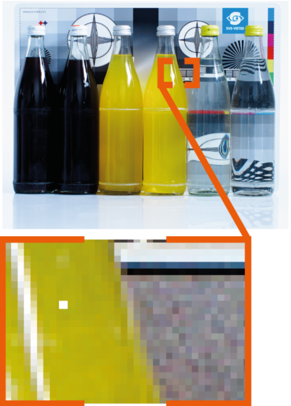
Fig. 5-22: Illustration of a defect pixel
