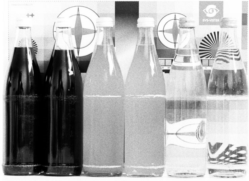
Fig. 5-1: Noise caused by too much gain
