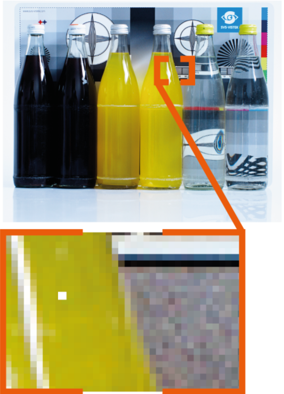
Fig. 5-27: Illustration of a defect pixel
