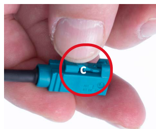
Figure 6: Pressing down the latch (c) of the FAKRA coaxial connector
